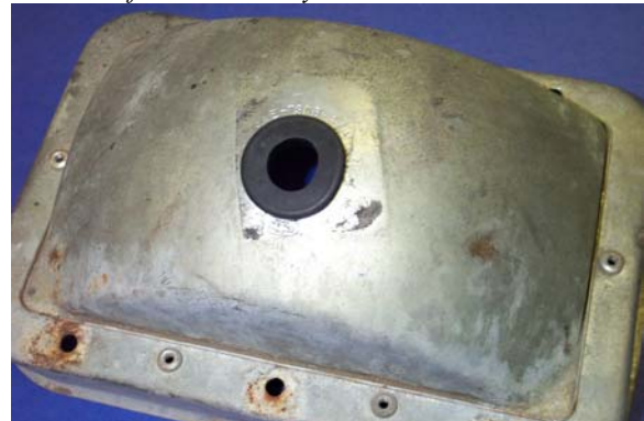
Rubber grommet installed in the taillight bucket.
