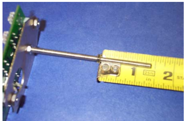
Position this nut 1-3/8" from the end of the screw.
