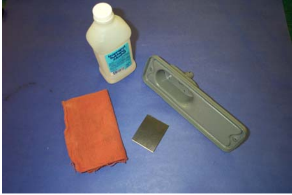
Locate the rubber insulating pad, wipe area with rubbing alcohol before installing.
