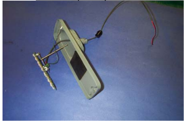
Pass the harness through the taillight housing and the supplied wire guide. The wire harness goes through the smaller hole.
