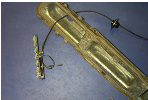
Pass the harness through the taillight housing and the supplied wire guide.
