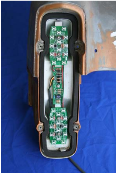
Install the provided taillight lens gasket on top of the LED bracket in the taillight housing.
