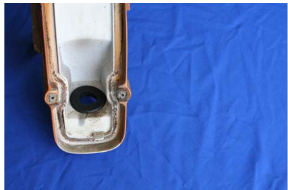
Install the provided rubber grommet in the old bulb hole.
