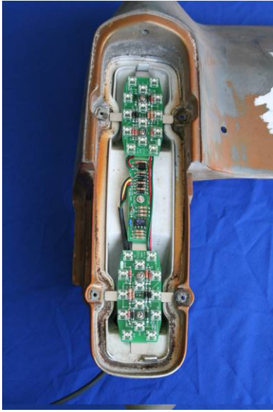
Install the LED bracket and array in the taillight housing.
