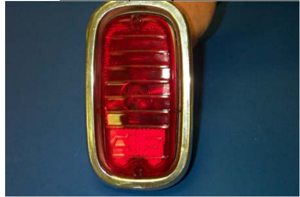
...and finally the lens. Install the lens screws and tighten. Don't over tighten!!
