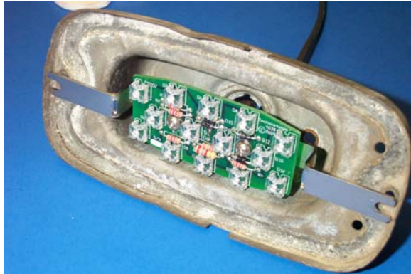
The slots in the end of the supplied stainless steel bracket aligns with the truck's lens screws.
