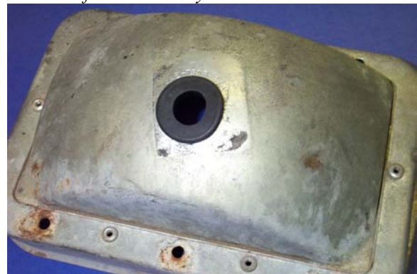
Rubber grommet installed in the taillight bucket.
