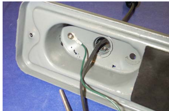
Install ground wire as shown. Be sure there is bare metal contacting the lug on the green wire. Very important!
