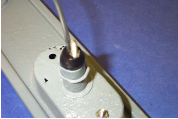
Install nut. Make sure the nut is tight enough so the LED array will not turn, but not tight enough to deform the LED array.
