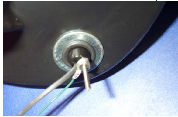
Attach the external grounding wire to the LED mounting stud.
