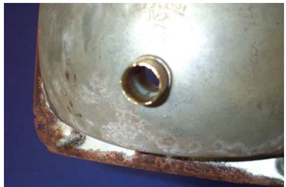
The bulb socket must be modified, as shown, to accept the supplied plastic wire guide.
