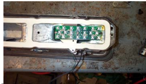
Install lens gasket on top of the stainless steel LED bracket.
